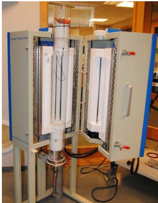
Fig 4. Photo of the type of furnace used in the Kjeller hot-cell LOCA tests.
