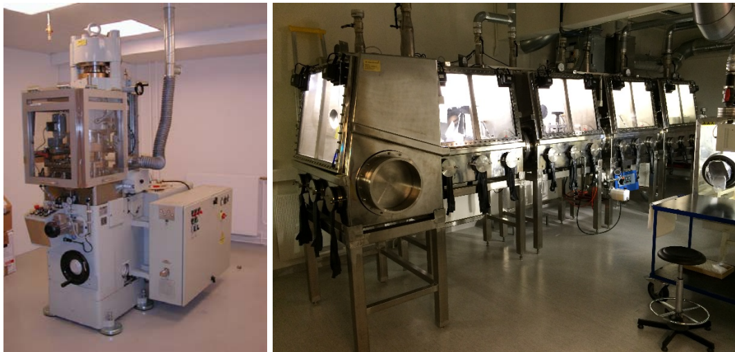
Fig 10. Left: \text{UO}_2 pellet press. Right: MOX and thorium fuel production line in glove boxes.
