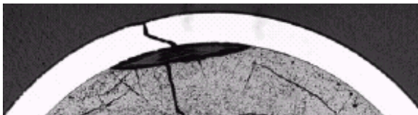
Fig. 1. Chipped pellet in fuel element with cracke cladding (with chip).
