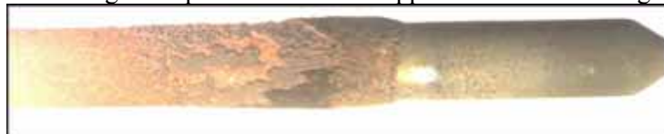
Fig. 3 A photo of the pre-cruded rod before autoclave exposure in phase 2C:1.
