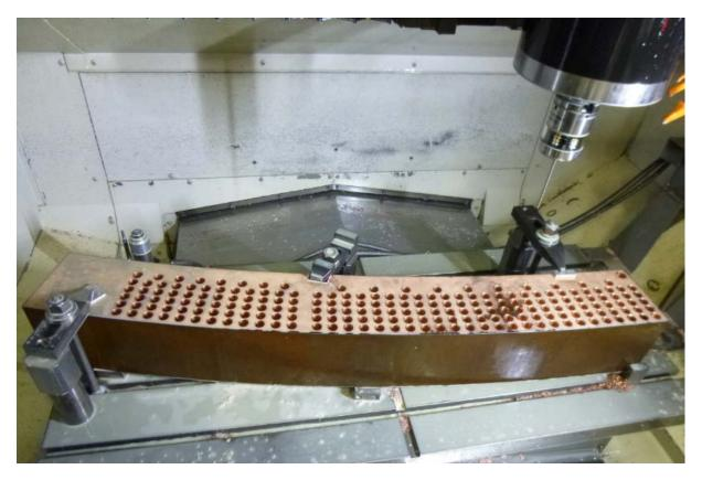
Fig.10 Heater segment with drilled holes.
