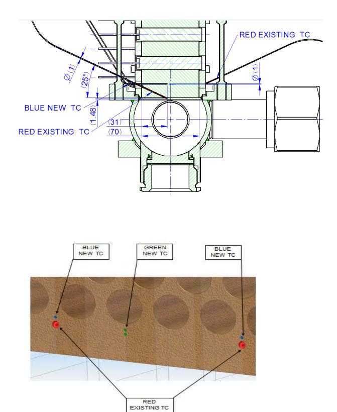
Fig.3. New thermocouple positions in the small scale sample.
