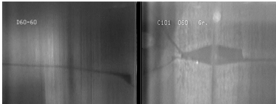
Fig. 2: Be channel with crack and with material loss (5 x 25 mm)
