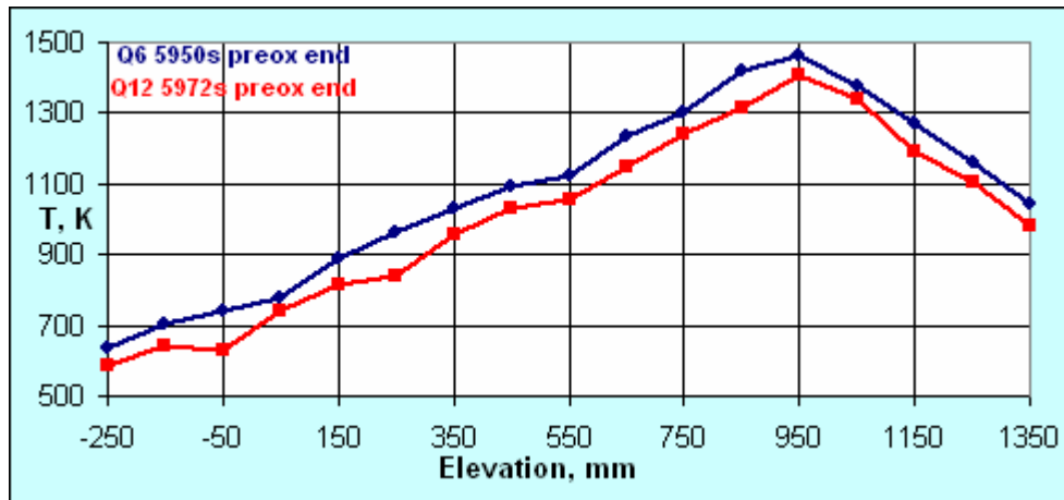
Figure 2: Axial temperature distribution at the end of pre-oxidation phase
