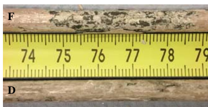
Figure 13: QUENCH-12, the withdrawn corner rods D and F revealed breakaway oxidation with intensive spalling of oxide scales
