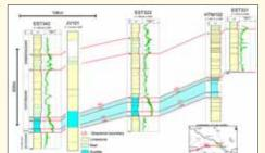
The mineralogical results for the various boreholes confirm the mineralogical composition of the host formation, which contains 30 to 55% clay minerals, associated with 20 to 30% carboacted 20 to 35% quartz and a small percentage of subordinate mineral 20 to 35% quartz and a small percentage of subordinate mineral carboacters.
