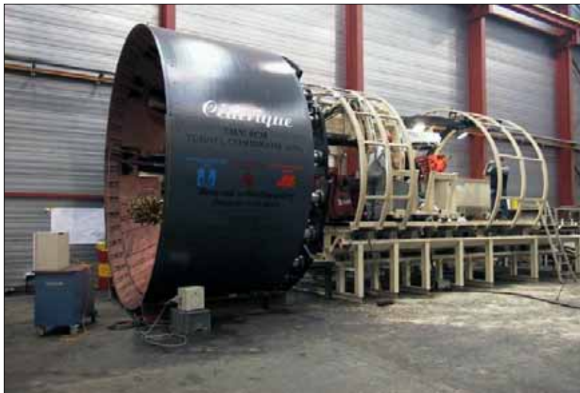
Fig 2. The tunnelling machine used for the construction of the connecting gallery
