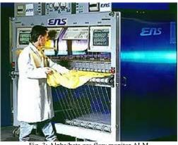
Fig. 3: Alpha/beta gas flow monitor ALM
