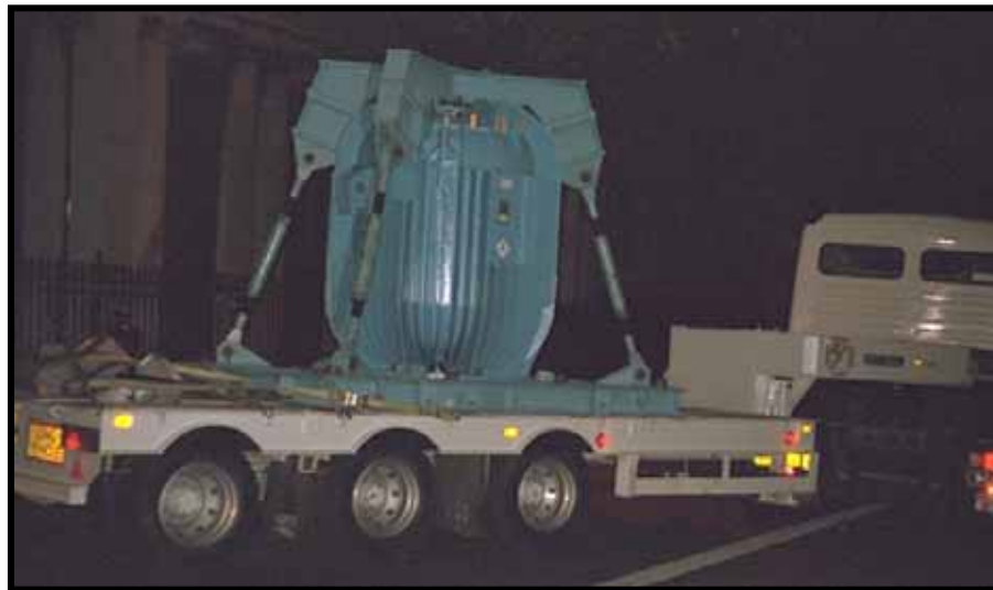
Fig 2. UNIFETCH Flask during transportation
