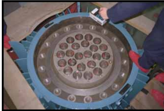
Fig 1. Open UNIFETCH Flask showing the baskets containing JASON Fuel
