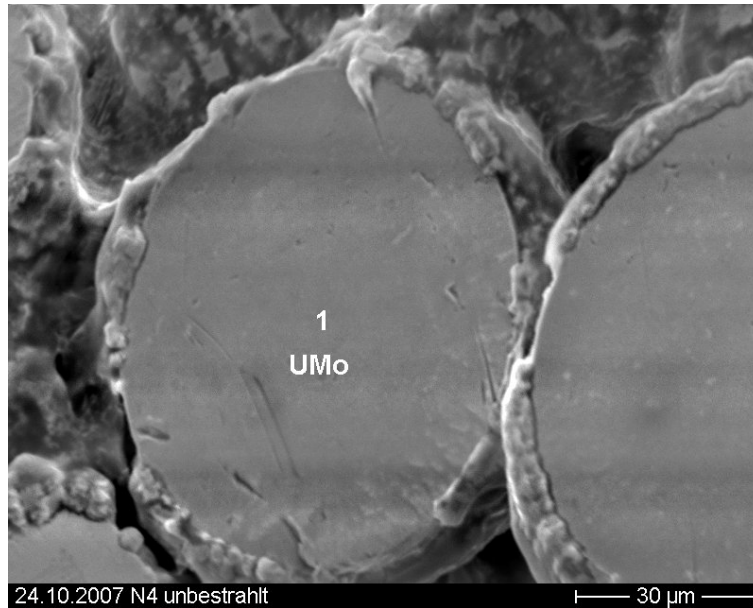
Fig. 6: SEM image of a not irradiated UMo grain. No IDL is visible. EDX data was taken on position 1, see Tab. 4.
