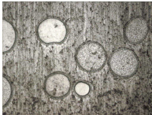
Fig. 1. Microstructure of the (U-9Mo-UO 2 )-Al tablets
