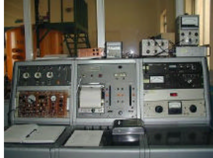
Fig. 3 Reactor Console of AGN-201, KHU
