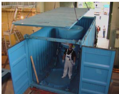
Figure 3: Loading Cask into ISO Container
