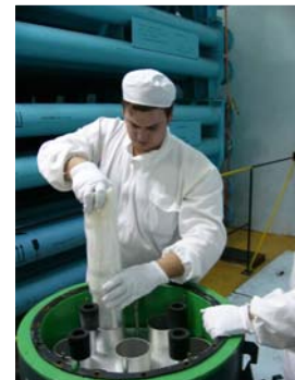
Figure 2: Loading IRT-2M HEU into Casks
