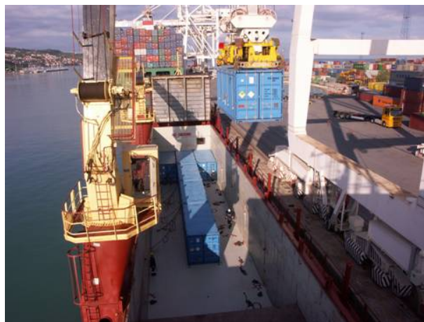
Fig.4. Loading the ship with the ISO containers
