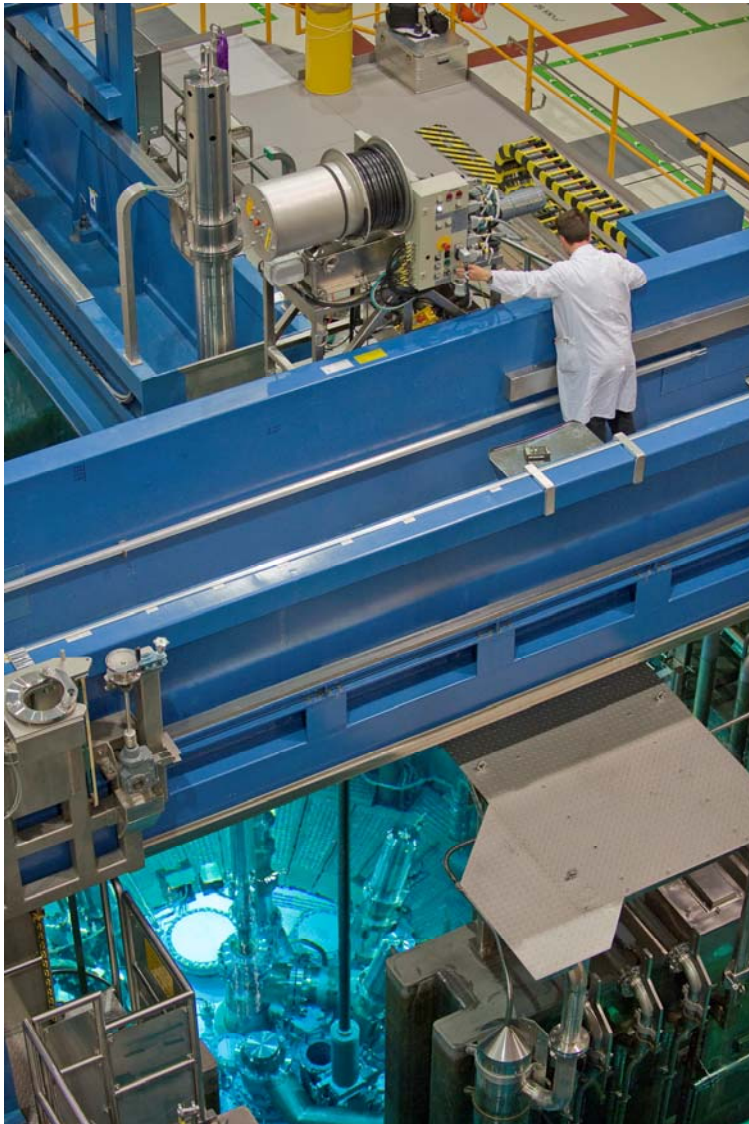
Figure 2: The Si doping facility is approaching the irradiation channel
