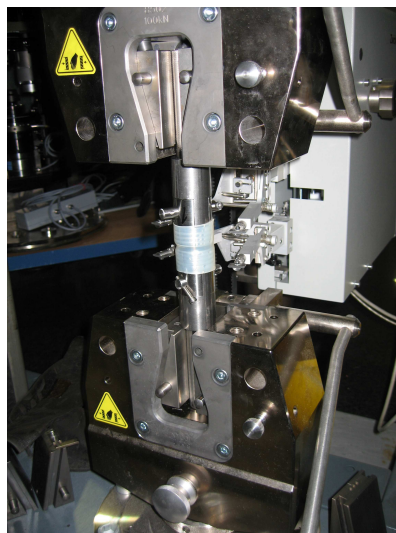
Figure 1: Tensile test machine with specimen holders
