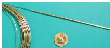
Figure 2: rhodium SPND for thermal neutron flux measurements (external diameter is 3mm)
