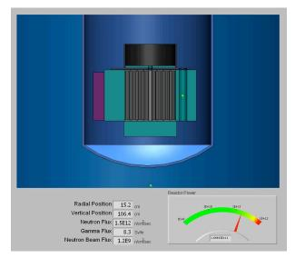
Figure 3: Flux map interface showing core profile
