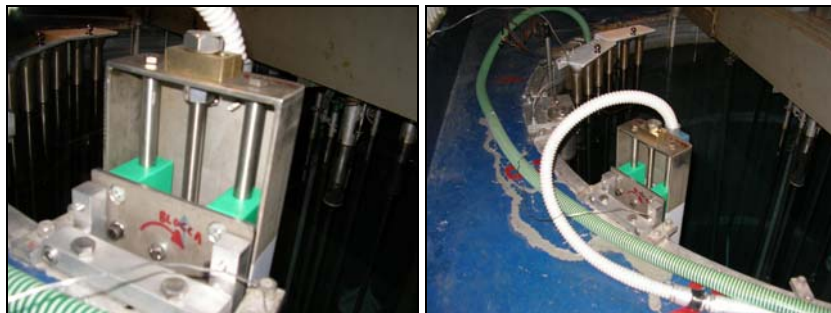
Fig. 2 – Ion chamber micrometric-positioning system detail
