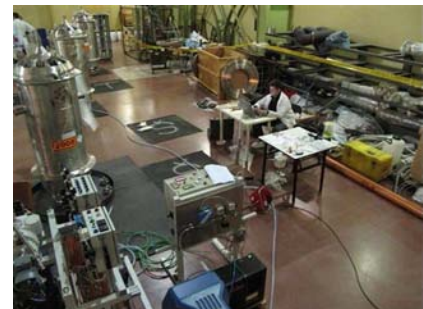
Fig 11. Drying and vacuuming of TUK-19 casks
