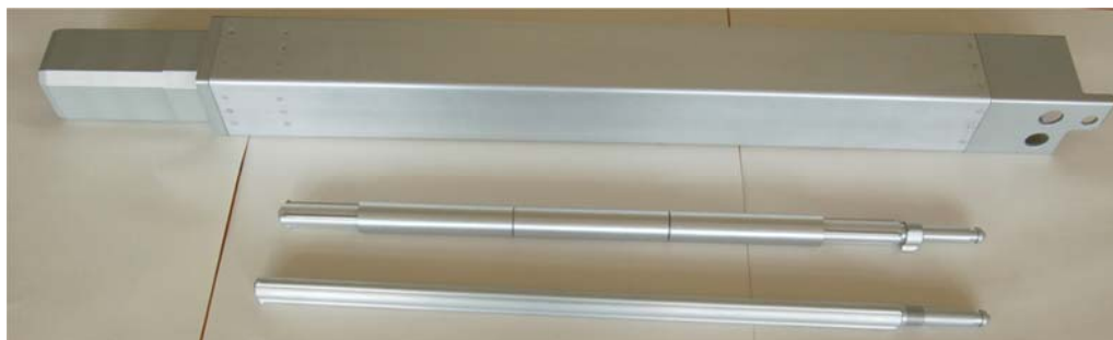
Fig.2 Irradiation device and target holder with 3 annular targets
