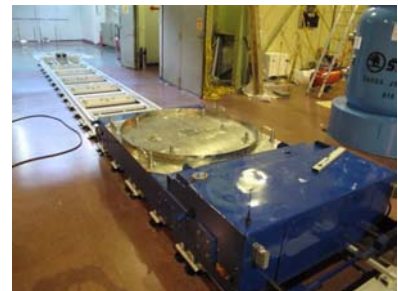
Fig 6. Cask rail-transfer device
