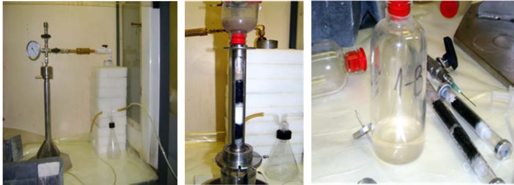
Fig.5 Images from dissolving and purification stages and final solution of sodium molybdate
