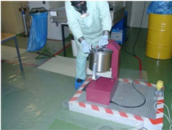
Fig 3. The special drum mixer for blending
