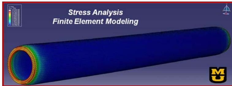
Fig. 1 ANL's LEU-foil annular target, thermal stress field
