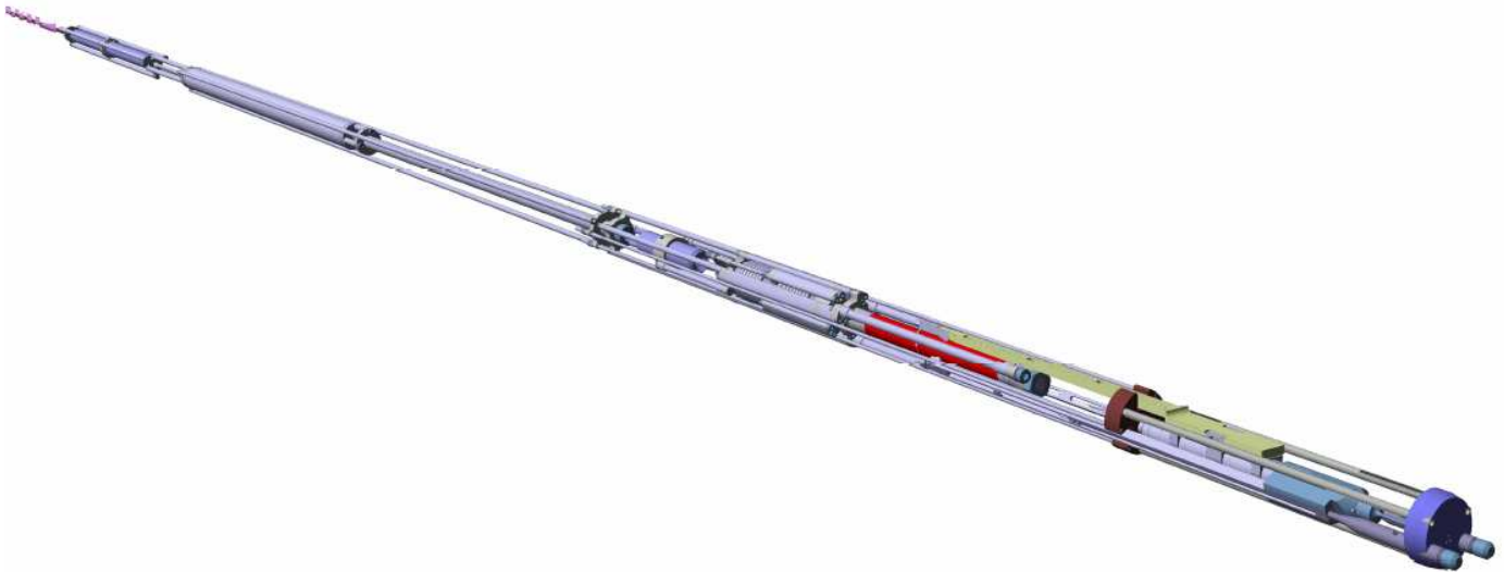
Figure 1. The lower part of the MeLoDIE sample holder showing from left: LVDT of mover, DG probe mover, specimen LVDT, bidirectional axial loading device, specimen and DG probe.
