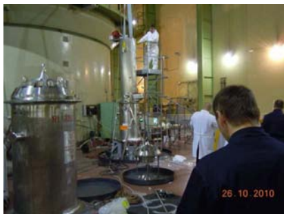
Fig 10. Loading a basket into TUK-19 cask
