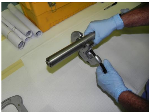
Fig. 1 - Cutting TRIGA rods at Oregon State
