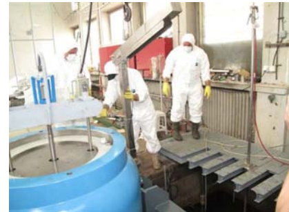
Fig 9. Loading a basket into SKODA cask
