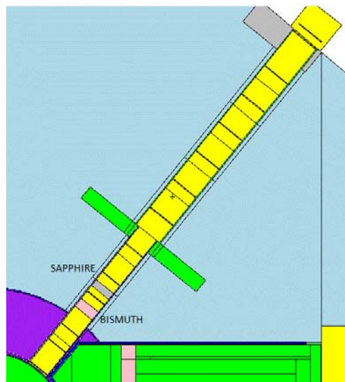
Fig 2. MCNP geometry for the channel B with the bismuth and sapphire filter inside.
