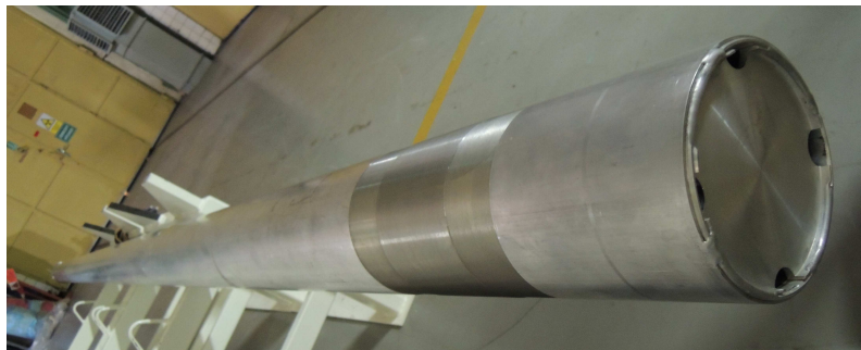
Fig. 7 Irradiation channel with shielding layer
