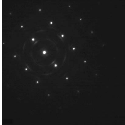
Figure 3: TEM micrographs from irradiated fuel showing a selective area diffraction pattern, z=[110] , where the anticipated BCC U-Mo crystalline structure is observed.
