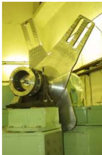
Fig. 2. A photo of the reactivity modulator rotors with nickel alloy blades at a test stand.
