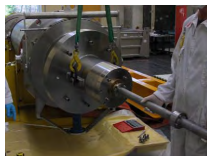
Figure 4 – Guillotine system and clock for plug removal
