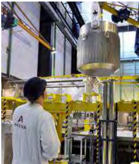
Fig.11: Cask handling to the preparation cell, before unloading © AREVA
