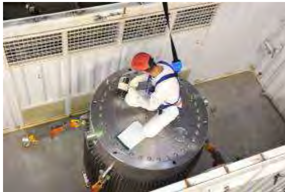
Fig.10: Radiological control on RRSF transportation cask, without shock absorber © AREVA
