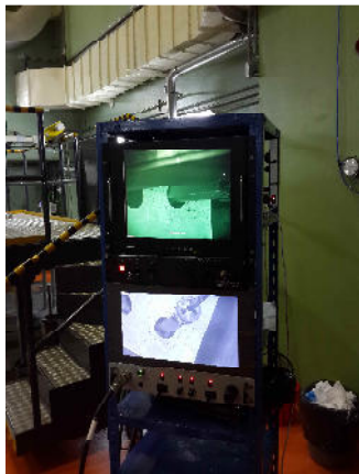
Fig. 4: Underwater camera systems used in FACIRI. To the right, view of fuels stored in a basket.
