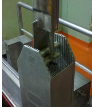
Fig. 7: Testing of the grappling tool for standard type MTR fuel and fuel isolation cans.
