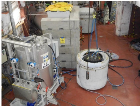
Figure 4: Resin transfer set-up with shielded containers
