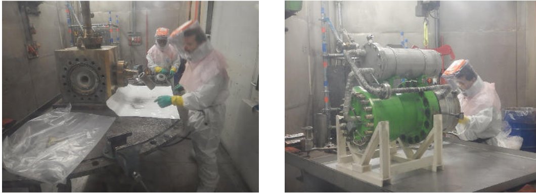
Figure 6: Material processing in the cutting and size reduction workshop at BR3
