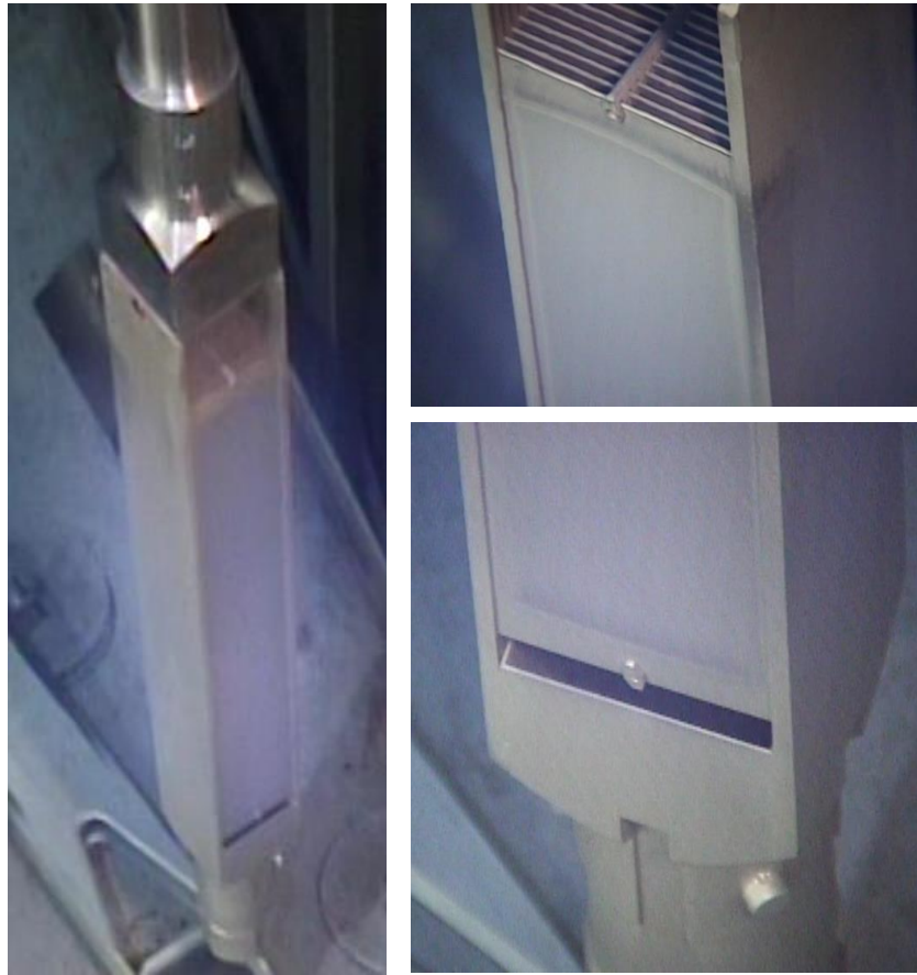
Figure 5 Visual inspection of the LTA after completion of 4 cycle irradiation
