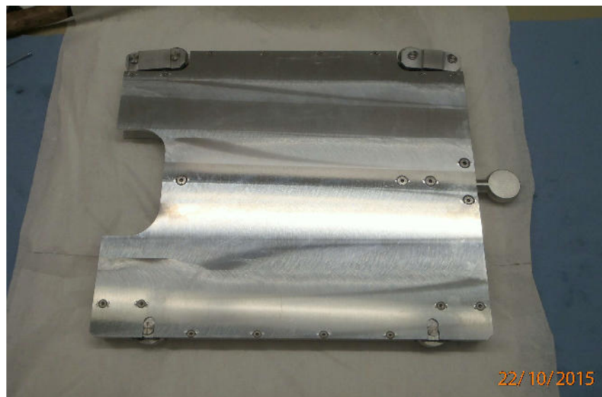
Fig 3. The new mobile carrier containing fresh fuel plates
