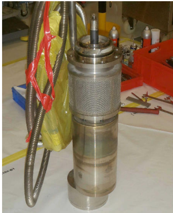
Fig 9. Canned motor pump of the converter facility
