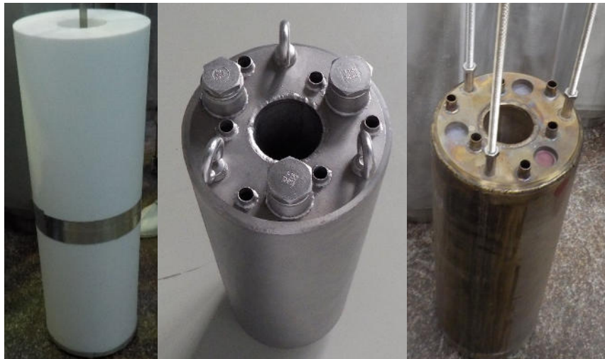
Figure 4, Photographs of used insertions (from left Teflon, canister with LiF-BeF 2 , canister with lead)
