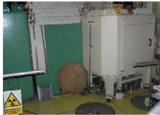
Fig. 2 Irradiation box at the HK1 beam
