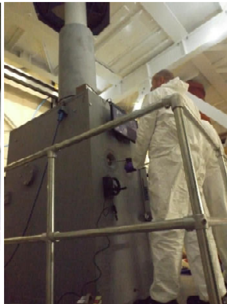
Figure 10: Cropper Shielded Cell aligned under flask way. The access door for transport container is open. The transport container is moved in and out of the cell on a trolley.
