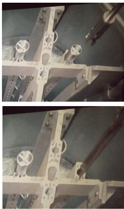
Figure 9b: Grab tool about to be connected to the 'end cap' lifting attachment and control rod blade being lifted out of the lower guide
