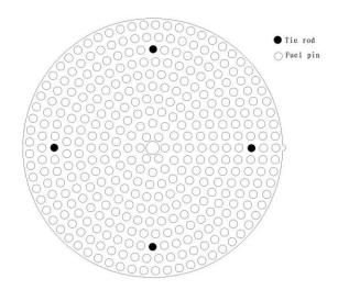
Fig. 2 The diagram of fuel arrangement
