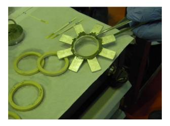
Fig 1. Coupons of AA6061 exposed to the water of a nuclear irradiated fuel storage facility.
