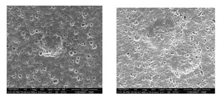
Fig 4. Example of corrosion under biofilm-oxide patches.
