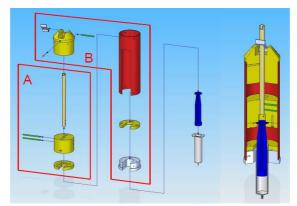
Fig 2. Sampler for taking sterile microbiological samples. (a) mobile (b) fixed
